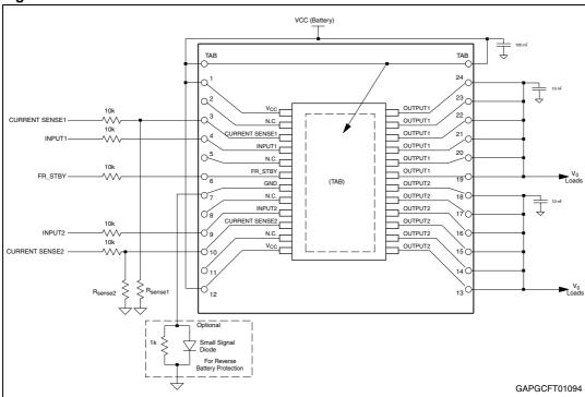
Figure 2. VND5T035AK evaluation board
