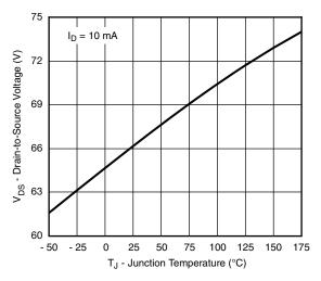
Drain Source Breakdown vs. Junction Temperature
