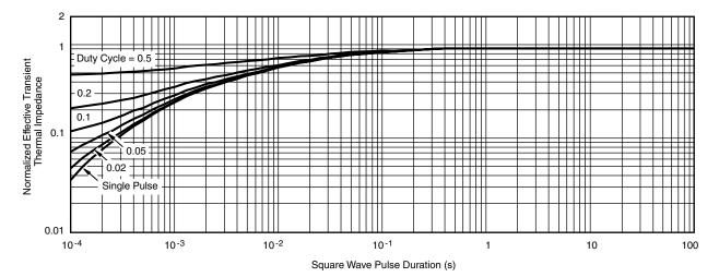
Normalized Thermal Transient Impedance, Junction-to-Case
