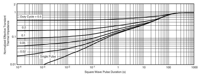
Normalized Thermal Transient Impedance, Junction-to-Ambient
