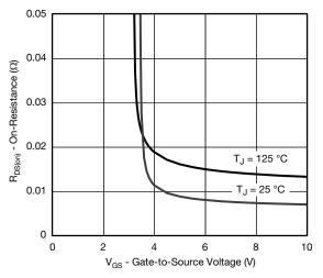
On-Resistance vs. Gate-to-Source Voltage
