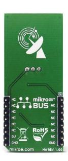
**Microwave click** detects movement, thanks to the PD-V11 a 24GHz microwave motion sensor. The typical use for Microwave click is a proximity or motion detector in various applications and devices.
