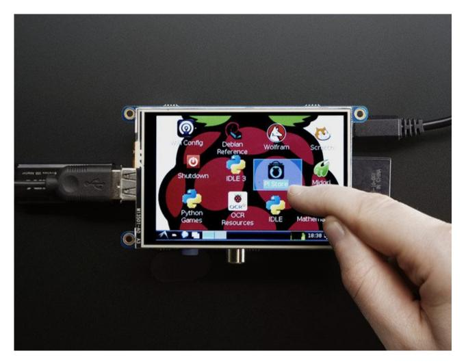
Is this not the cutest, little display for the Raspberry Pi? It features a3.5" display with 480x320 16-bit color pixels and a resistive touch overlay, but is only slightly larger than our popular original (http://adafru.it/dDE). The plate uses the high speed SPI interface on the Pi and can use the mini display as a console, X window port, displaying images or video etc. Best of all it plugs right in on top!
