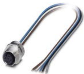
Sensor/Actuator flush-type socket, 5-pos., M12, A-coded, front/screw mounting with M16 thread, with 1.5 m TPE litz wire, 5 x 0.34 mm 2
