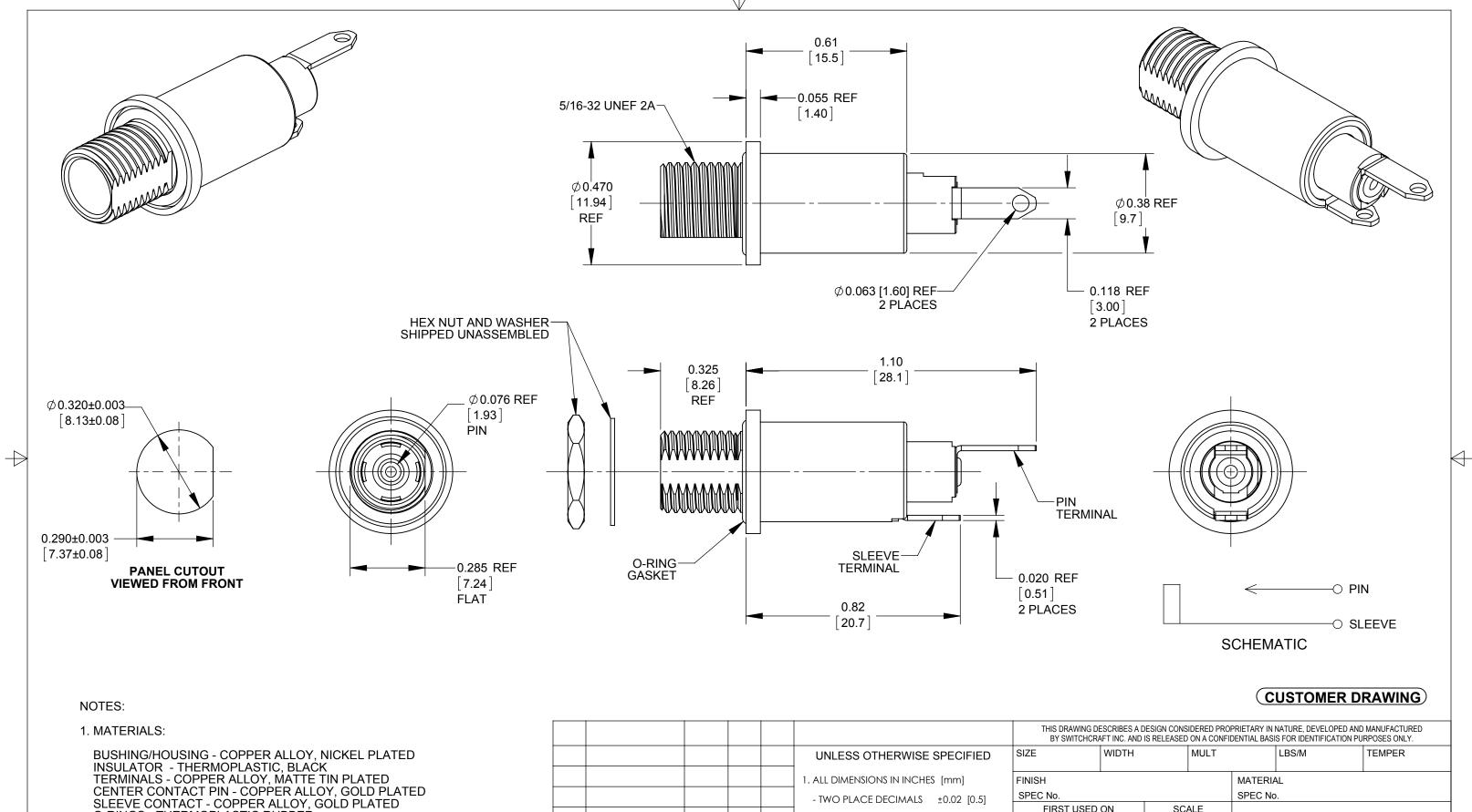
BUSHING/HOUSING - COPPER ALLOY, NICKEL PLATED INSULATOR - THERMOPLASTIC, BLACK TERMINALS - COPPER ALLOY, MATTE TIN PLATED CENTER CONTACT PIN - COPPER ALLOY, GOLD PLATED SLEEVE CONTACT - COPPER ALLOY, GOLD PLATED O-RINGS - THERMOPLASTIC RUBBER HEX NUT - COPPER ALLOY, NICKEL PLATED WASHER - STEEL, NICKEL PLATED
