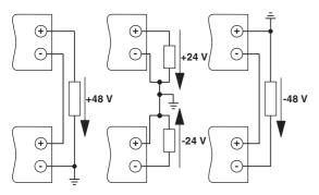
Figure 29 Schematic diagrams in series operation
