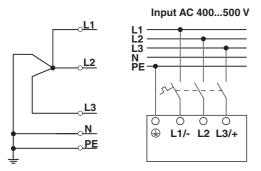
Figure 14 Pin assignment for AC supply voltage
