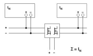
Figure 31 Schematic diagram, redundant operation with QUINT ORING
