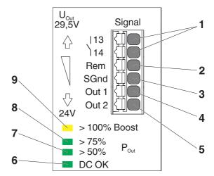
Figure 23 Position of the signaling element
