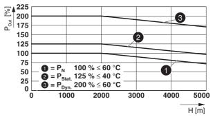
Figure 35 Output power depending on the installation height
