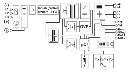
Figure 6 Block diagram
