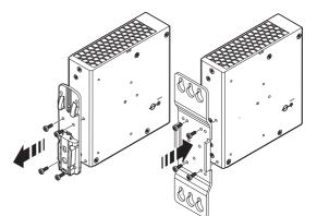
Figure 11 Mounting the UWA 182/52 universal wall adapter
