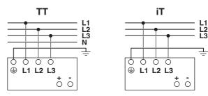
Figure 13 Network configurations in star network
