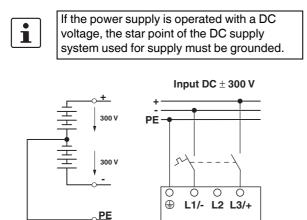
Figure 15 Pin assignment for DC supply voltage
