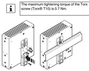
Figure 10 Mounting the universal DIN rail adapter
