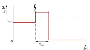
Figure 18 FUSE MODE output characteristic curve
