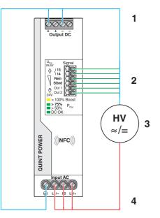
Figure 1 Potential-related wiring for the high-voltage test
