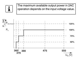
Figure 34 Output power in 2AC operation
