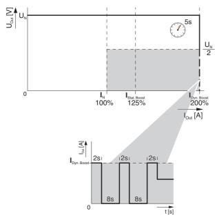
Figure 17 Smart HICCUP output characteristic curve
