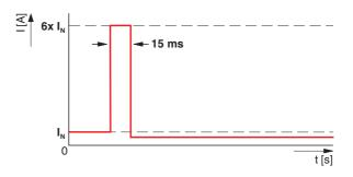
Figure 21 SFB pulse trips circuit breakers
