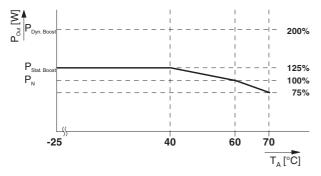
Figure 33 Output power depending on the ambient temperature
