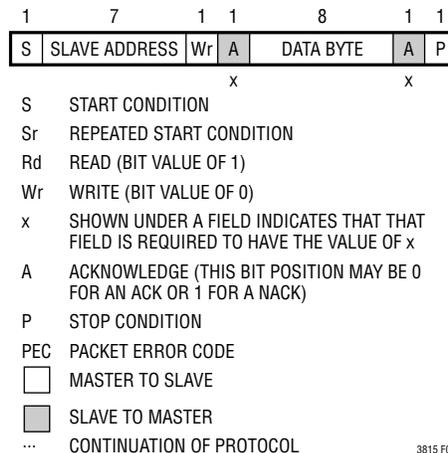
Figure 2. PMBus Packet Protocol Diagram Element Key
