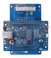
Plug the Aptina Image Sensor Board into the Aptina Image Sensor Interconnect Board (The Aptina Image sensor board is not part of this kit)
